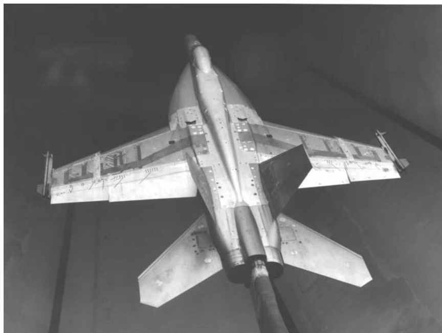
Figure 1 : F/A-18E model installed in LaRC 16-Foot Transonic Tunnel.
